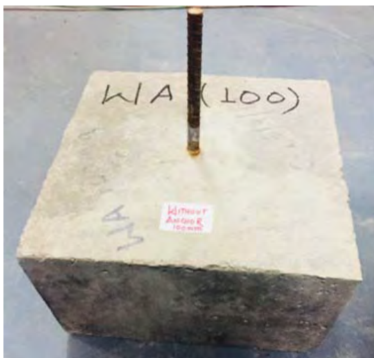
Headed Bar Embedded in Concrete Cube
