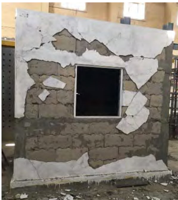
Damage Pattern from Lateral Load Test
