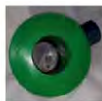
Shows that the Inside portion of the bedding is covered with barrel of WPE55 Pipe Collar
