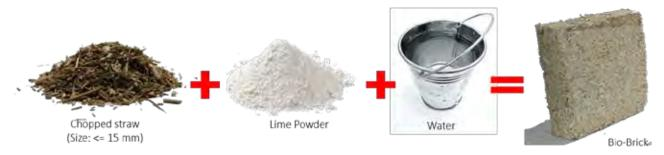
Bio-brick is prepare by mixing chopped husk, lime slurry in 1:3 ratio by weight.
