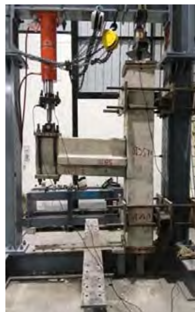
Cyclic Load Test Set-up
