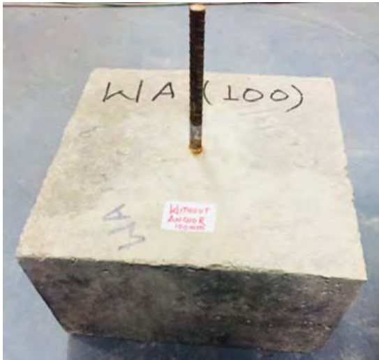
Headed Bar Embedded in Concrete Cube
