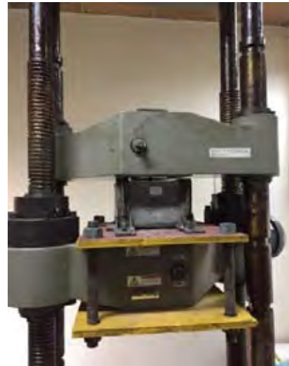
Pull-out Test Set-up
