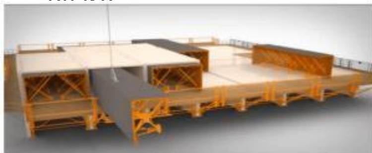
Box out of door and windows
