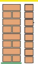
230 mm + 40 mm cavity +115 mm brick with U value – 1.1 w/ m<sup>2</sup>k
