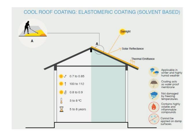
Elastomeric Coating Solvent & Water based
