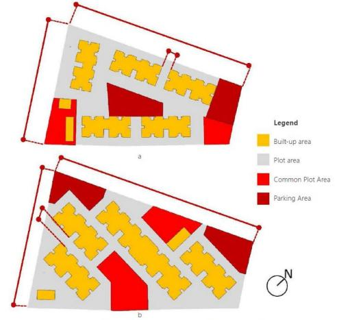
**Figure 142:** (a)- Site plan for case 1; (b) Site plan for case 2 and 3 Reorientation and rearrangements of blocks.
