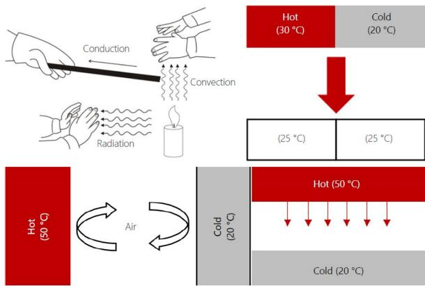
Clockwise- Forms of heat transfer; Conduction; Radiation; Convection Source- https://thefactfactor.com/facts/pure\_science/physics/conduction/9868/; Rawal, R., 2021. Heat Transfer and Your Building Envelope, Solar Decathlon India
