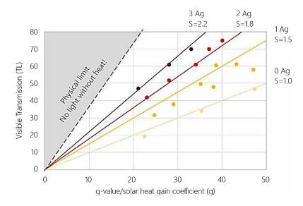
Selectivity, solar heat gain coefficient and visible light transmission of different low e-coating combinations
