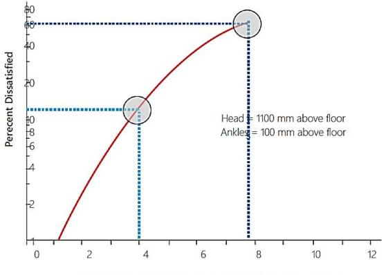
Air Temperature Difference between Head and Ankles °C
