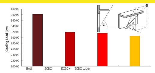
Cooling loads for BAU, ECBC, ECBC+, and ECBC super buildings having 600mm shading over windows
