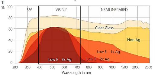
Performance of different low-e coating combinations in UV, visible light, and IR spectrums.
