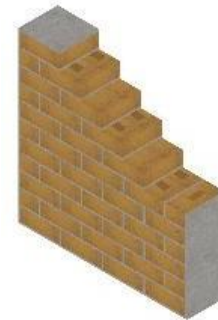
Unstabilized Adobe U - VALUE ( \text{W/m}^2 \text{K} )= 1.57
