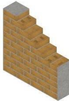
AAC block wall U - VALUE ( \text{W/m}^2 \text{K} )= 0.45
