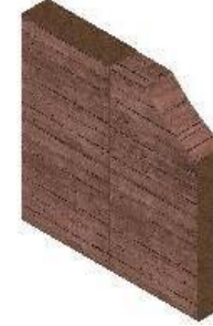
Stabilized Rammed Earth Wall assembly U - VALUE ( \text{W/m}^2 \text{K} )= 1.495
