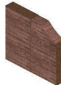
Unstabilized Rammed Earth Wall assembly U - VALUE ( \text{W/m}^2 \text{K} )= 1.68
