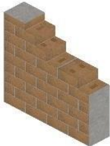
Compressed Stabilized Earth block wall U - VALUE ( \text{W/m}^2 \text{K} )= 1.59
