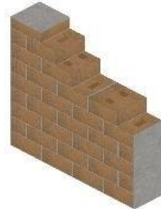
Unstabilized Compressed Earth block wall U - VALUE ( \text{W/m}^2 \text{K} )= 1.42
