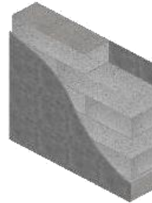
AAC block wall U - VALUE ( \text{W/m}^2 \text{K} )= 0.45
