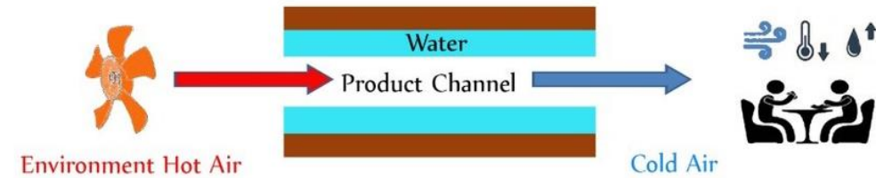
The Direct Evaporative Cooling System
