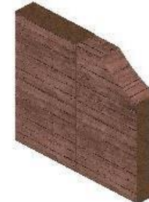
Unstabilized Rammed Earth Wall assembly
