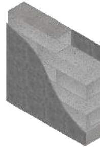
AAC block wall U - VALUE (W/m 2 K)= 0.45
