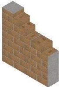
Compressed Stabilized Earth block wall U - VALUE (W/m 2 K)= 1.59
