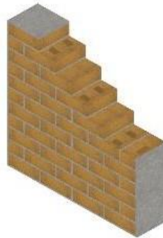
AAC block wall U - VALUE (W/m 2 K)= 0.45
