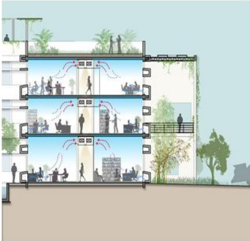
OFFICE – Active cooling system
