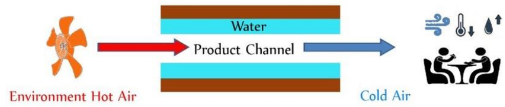
The Direct Evaporative Cooling System
