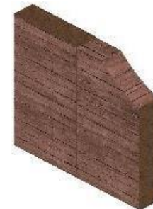
Unstabilized Rammed Earth Wall assembly U - VALUE (W/m 2 K)= 1.68
