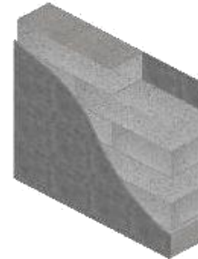
AAC block wall U - VALUE (W/m 2 K)= 0.45
