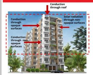
To limit the heat gain/loss from the building envelope, the code specifies:
