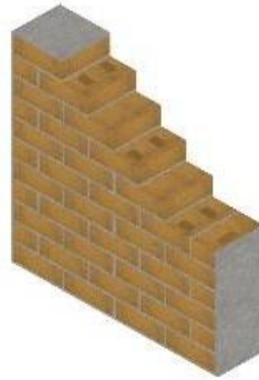
AAC block wall U - VALUE (W/m 2 K)= 0.45
