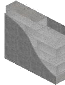
AAC block wall U - VALUE (W/m 2 K)= 0.45
