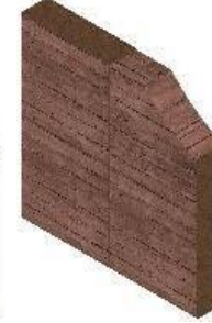
Stabilized Rammed Earth Wall assembly U - VALUE (W/m 2 K)= 1.495
