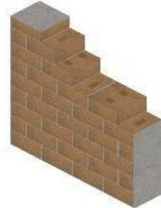
Unstabilized Compressed Earth block wall U - VALUE (W/m 2 K)= 1.42
