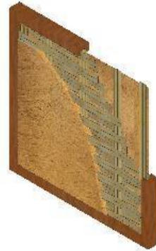
Unstabilized Compressed Earth block wall U - VALUE (W/m 2 K)= 1.42
