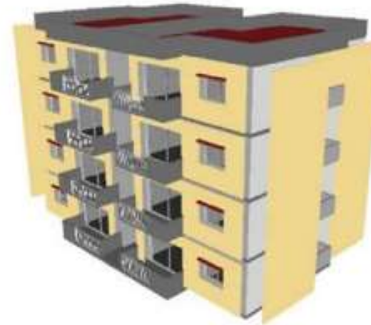
RETV - 18.0 W/m 2 Building Envelope Details: Better insulation in walls and roof (U-value) High solar reflectance on roof (SRI)
