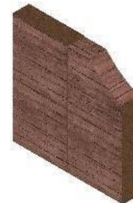
Unstabilized Rammed Earth Wall assembly U - VALUE ( \text{W/m}^2 \text{K} )= 1.68
