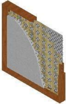
Bamboo-Crete U - VALUE ( \text{W/m}^2 \text{K} )= 1.82
