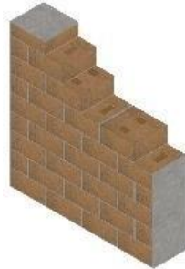
Unstabilized Compressed Earth block wall U - VALUE ( \text{W/m}^2 \text{K} )= 1.42
