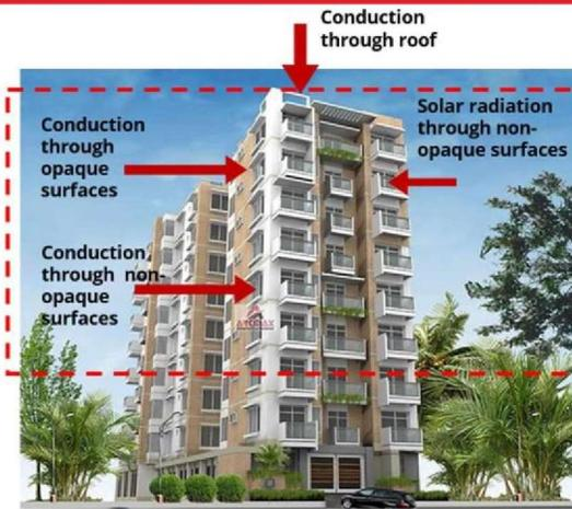
To limit the heat gain/loss from the building envelope, the code specifies:
