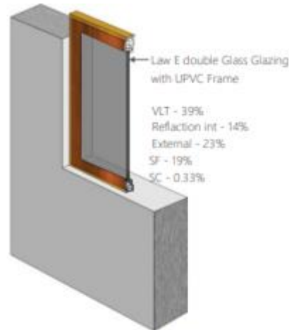
WINDOW U-value ( W/m^2K ) = 1.70 R-value ( m^2K/W ) = 0.588
