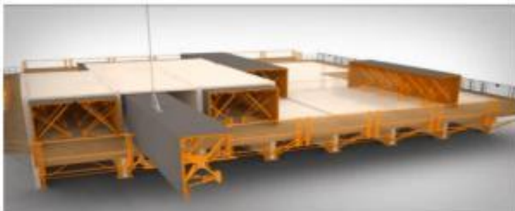
Box out of door and windows
