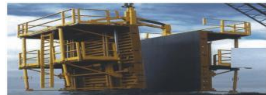
Monolithic Tunnel Formwork Panel
