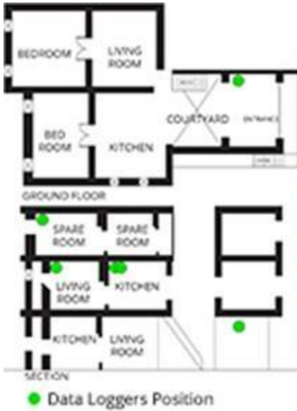
Plans of Pol House (PH) and Conventional House (CH) with data logger positions (green dots) and photographs
