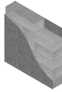
AAC block wall U - VALUE (W/m 2 K)= 0.45
