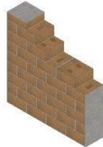
Unstabilized Compressed Earth block wall U - VALUE (W/m 2 K)= 1.42
