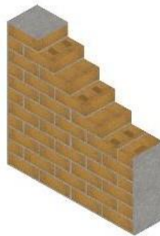
AAC block wall U - VALUE (W/m 2 K)= 0.45
