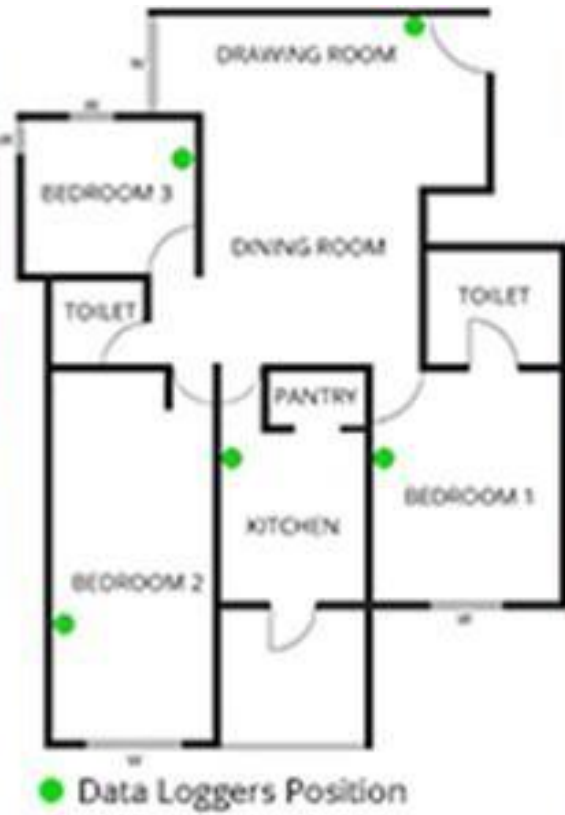
Plans of Pol House (PH) and Conventional House (CH) with data logger positions (green dots) and photographs
