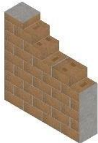
Compressed Stabilized Earth block wall U - VALUE (W/m 2 K)= 1.59
