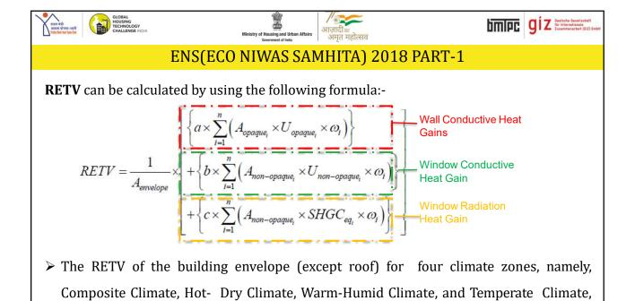
shall comply with the maximum RETV of 15 W/m<sup>2</sup>
