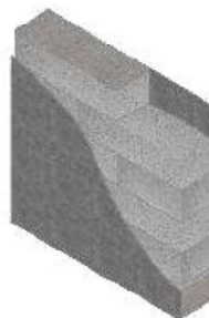
AAC block wall U - VALUE ( \text{W/m}^2\text{K} )= 0.45
