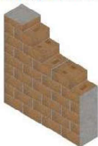
Compressed Stabilized Earth block wall U - VALUE ( \text{W/m}^2\text{K} )= 1.59
