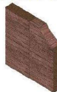
Unstabilized Rammed Earth Wall assembly U - VALUE ( \text{W/m}^2\text{K} )= 1.68
