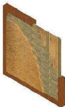
Unstabilized Compressed Earth block wall U - VALUE ( \text{W/m}^2\text{K} )= 1.42
