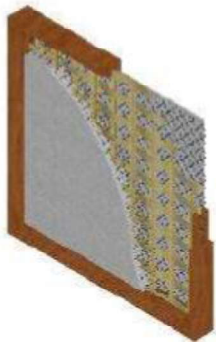
Compressed Stabilized Earth block wall U - VALUE ( \text{W/m}^2\text{K} )= 1.59
