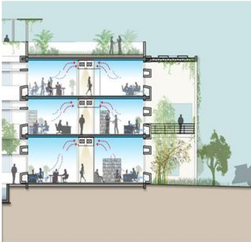
OFFICE – Active cooling system
