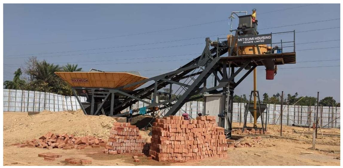
To bring resource efficiency, optimization of building materials and for quality control, a computerized batching plant has been established at site.
