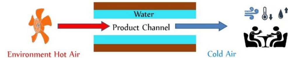
The Direct Evaporative Cooling System
