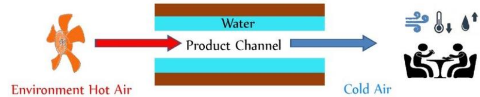
The Direct Evaporative Cooling System
