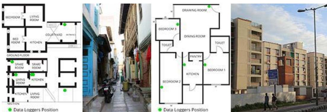
Figure 130: Plans of Pol House (PH) and Conventional House (CH) with data logger positions (green dots) and photographs
