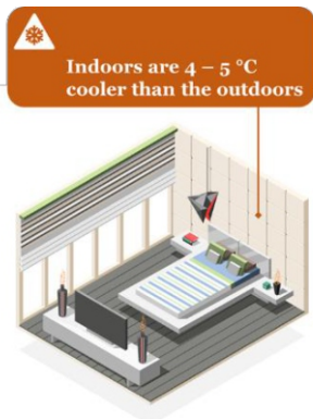
Figure 3: During the daily day & night cycle over a week in the monsoon month, 98% of the time the indoor temperature stayed within the IMAC comfort band
