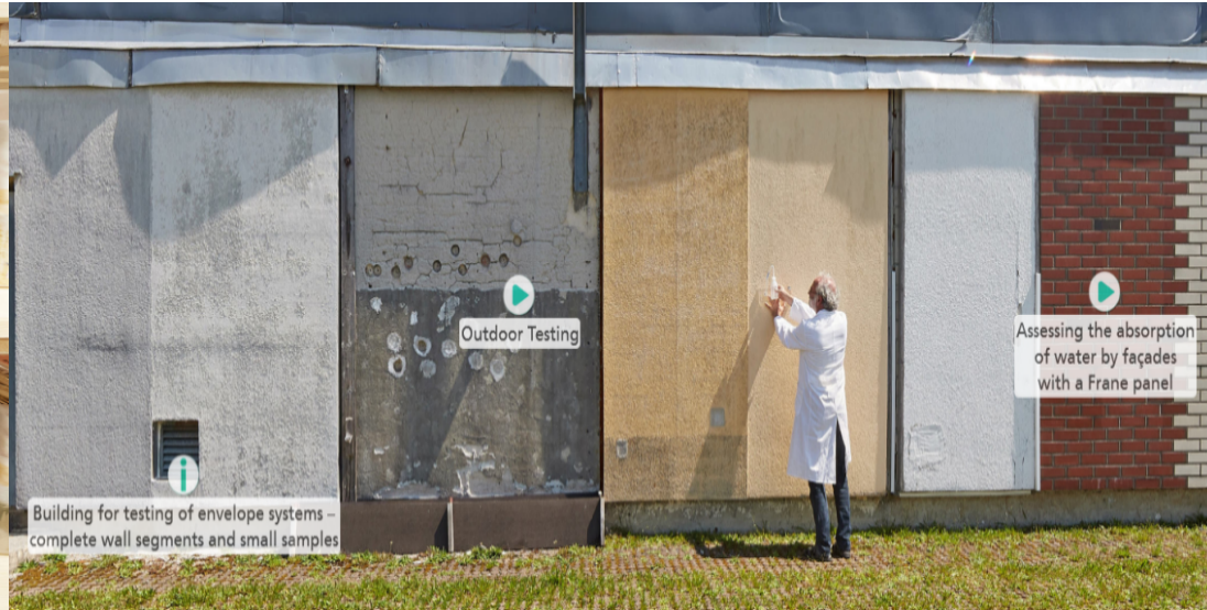
Free field testing of exterior walls
