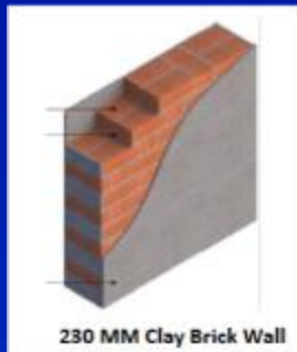
230 MM Clay Brick Wall
