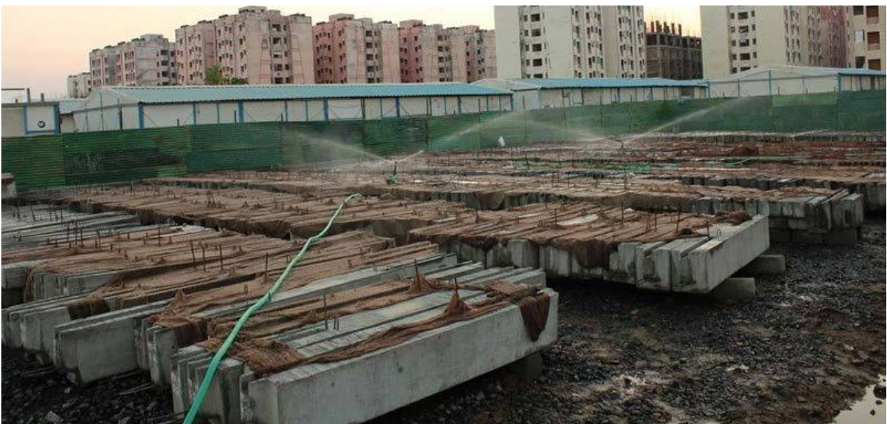
Curing on Manufactured Precast Beams
