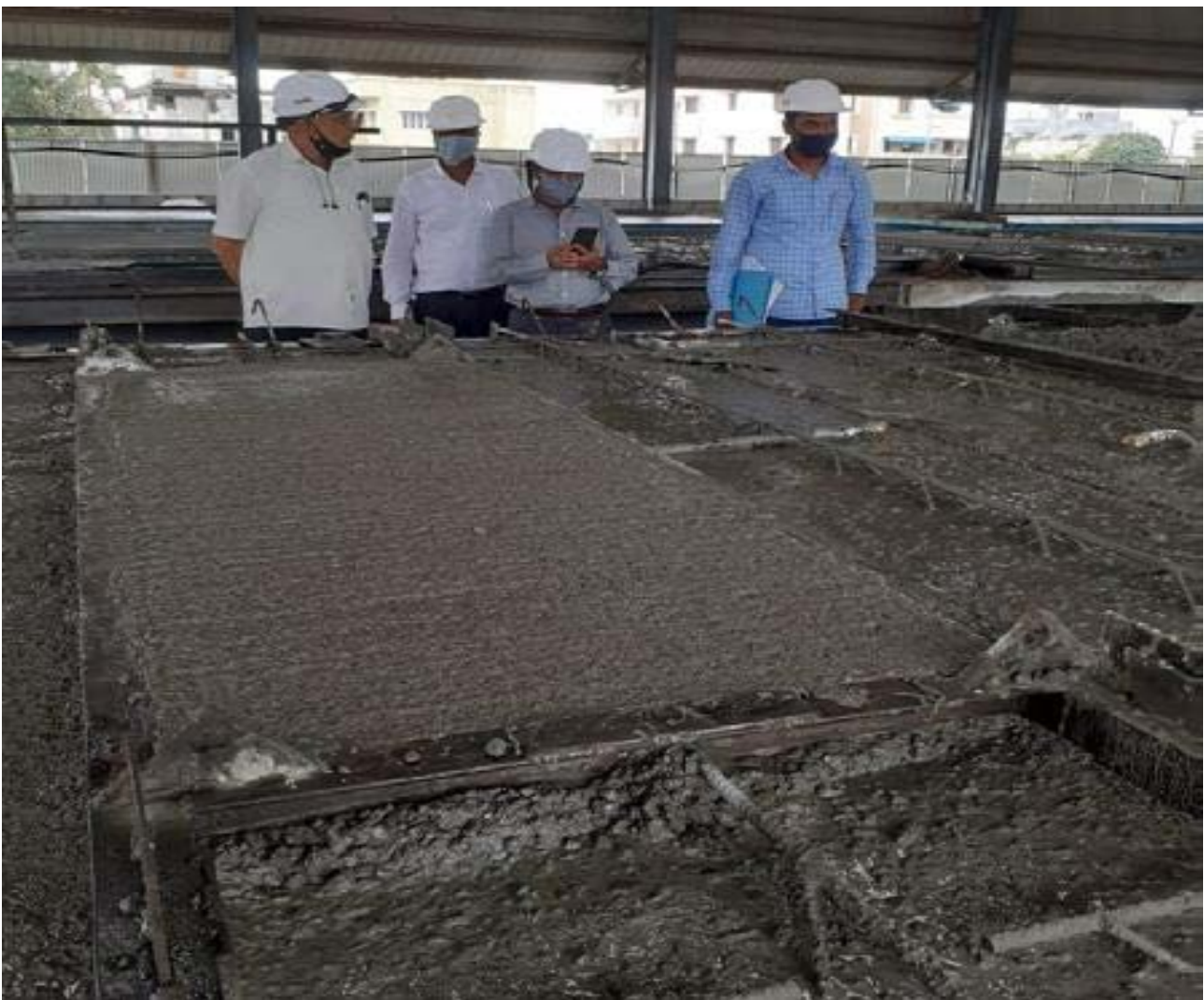
Manufacturing of Precast Slab
