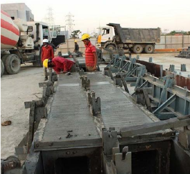
Manufacturing of Precast Columns
