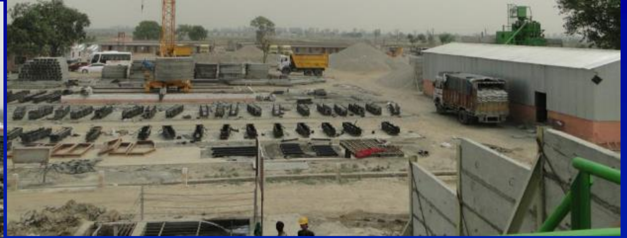
Precast yard and factory set-up at Delhi
