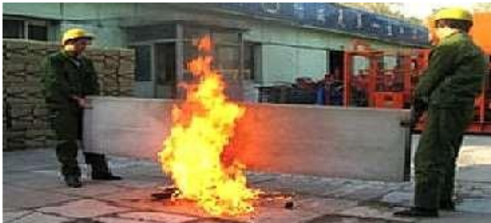
Fire Resistance Test
