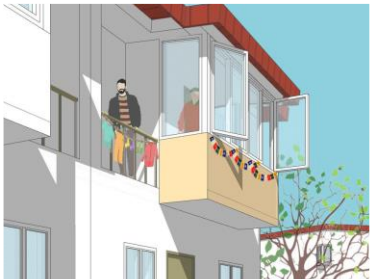
Sun balcony on south facade to trap maximum heat inside.
