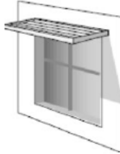
Use louvers in place of solid overhang for more light while still shading
